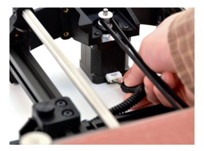
**5B** Remove and discard packaging tape securing Y-axis cable bundle.
