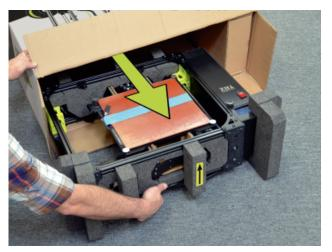
**2B** Carefully remove the protective foam piece that is supporting the Y-axis assembly.
