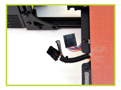
**5D** Connect the three sets of corresponding wire connectors, as shown below.
