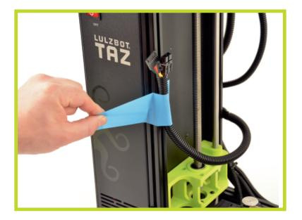
**5C** Locate the three cables found on the left side of the print surface.
