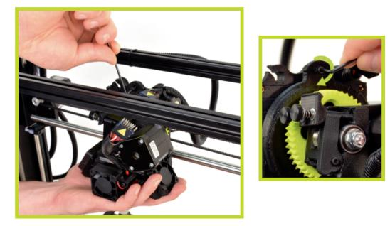
**7C** Reinsert and tighten the tool head mounting screw clockwise with the 2.5mm hex key to secure the tool head. Support the tool head with your hand to prevent it from falling onto the print surface.
