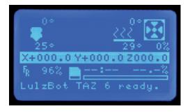
*If your Graphical LCD controller shows any error messages or does not seem to power on properly, unplug the printer and then check all connections made in previous steps. Visit LulzBot.com/Support for more assistance.*
