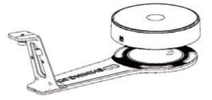
2) Screw the scanner into the socket on the stand.
