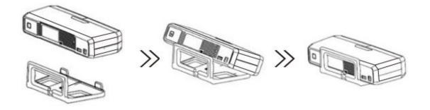
• Step 2. Insert calibration board onto the board holder . NOTE : Rotate the calibration board only while calibration.
