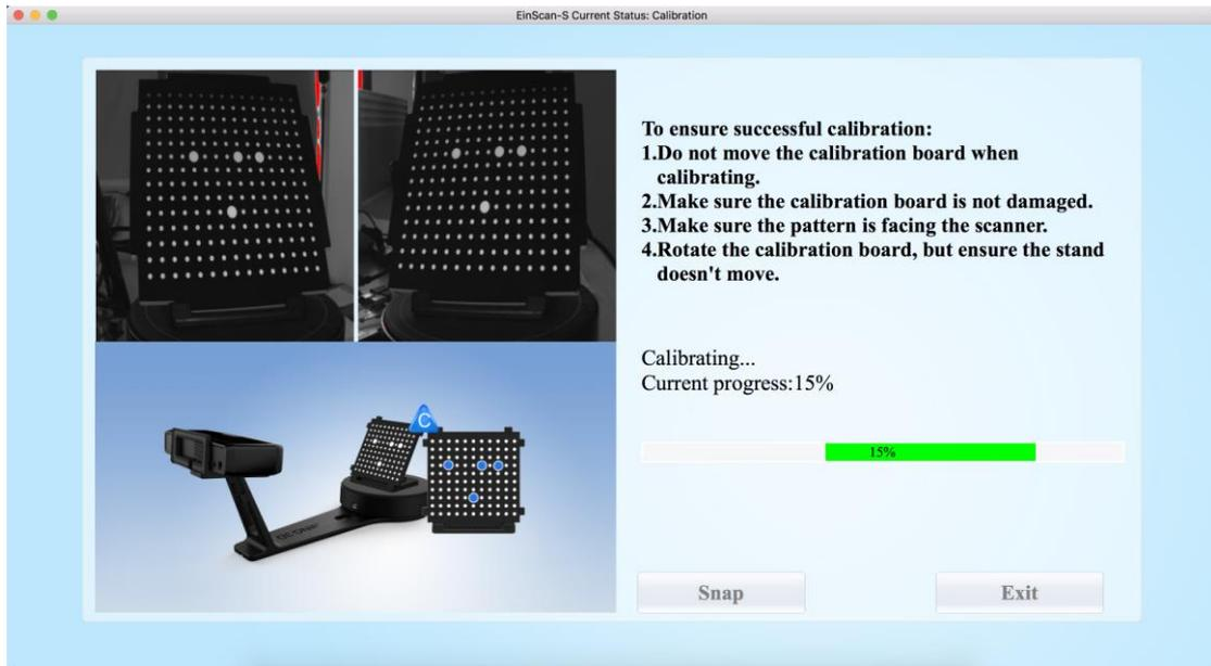
When calibration is finished, the software will close the calibration window automatically and enter the scan mode selection page.
