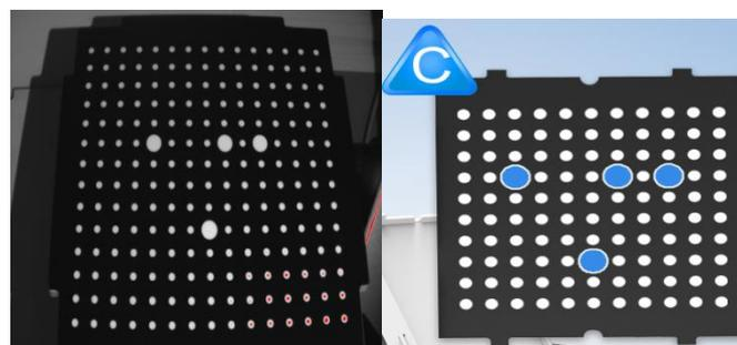
Upon completion of the 3rd calibration sequence, the software will automatically calculate and archive the current conditions. This calculation may take several seconds but once complete, you are ready to start automatic turntable scanning.
