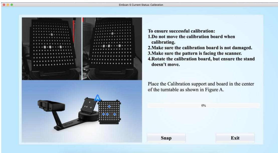
**Calibrating your scanner is important in order to get accurate scan results. The following describes the three steps required to successfully calibrate your scanner.**
