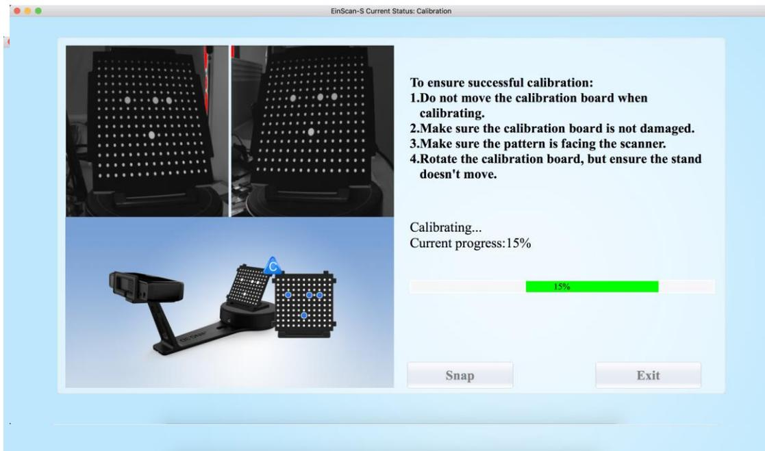
**⚠ Don't move the support. Only rotate the calibration board.**
