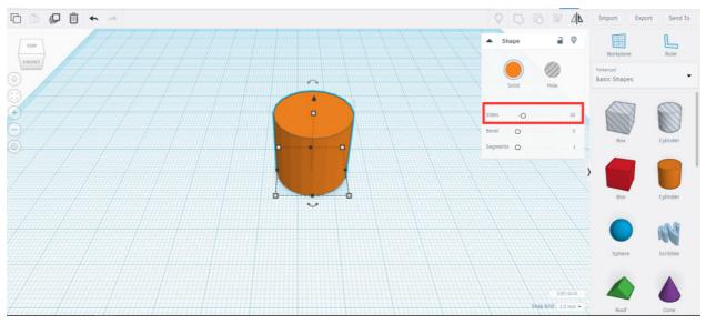
• The diameter of the axle hole at the bottom should be about 0.5mm larger than the axle.
