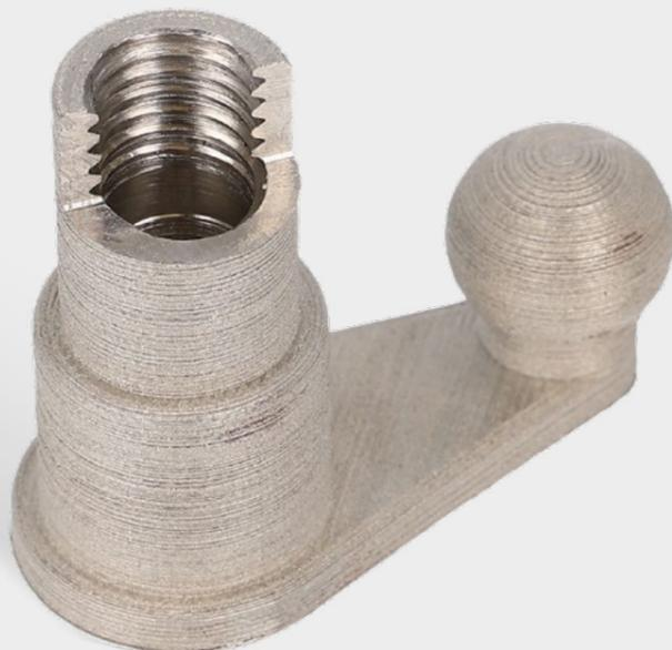
It is recommended to rework threaded holes regardless of printing direction or size. The diameter of the hole should be reduced to the diameter of the core hole so that the thread can then be re-tapped.
